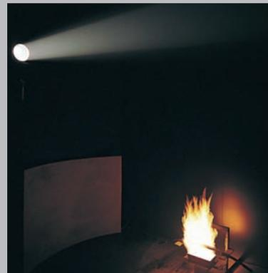
The test chamber is a 27 m<sup>3</sup> cube. The measurement system consists of a light source (100 Watt halogen lamp) and a silicon photo-electric-cell as the receiver. A tray filled with 1 liter of alcohol serves as the ignition source. A fan is used to ensure even smoke distribution with a metal screen protecting the tray from any flame turbulence. The alcohol is ignited and the light intensity of the photocell will be recorded.
