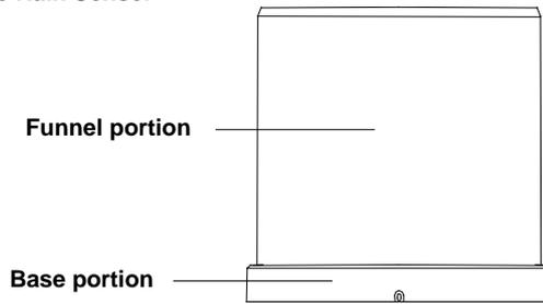
For best results, the rain sensor should be securely mounted onto a horizontal surface about 1 meter above the ground and in an open area away from trees or other coverings where rainfall may be reduced causing inaccurate readings.
