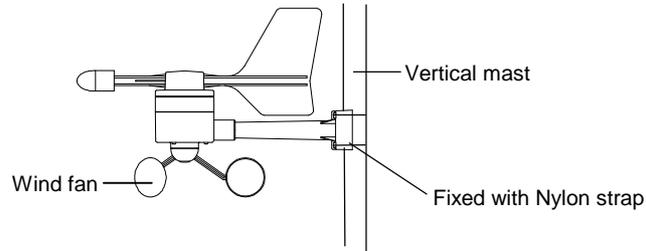
1. Unlock the mounting bracket from the remote wind speed sensor leaving the wire going through the bracket.
