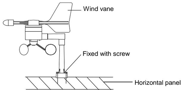
1. Unlock the mounting bracket from the remote wind speed sensor leaving the wire going through the bracket.
