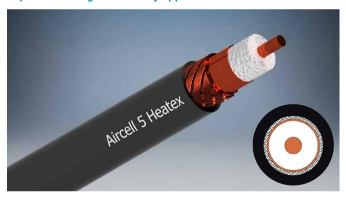
Aircell 5 Heatex is a flexible and thin coaxial cable with 5 mm outer diameter for the frequency range from DC to 10 GHz. Its low loss characteristics and the ability to use standard RG 58 connectors make this cable the number one choice not only for Wireless LAN applications but also for general RF communications.
