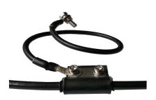
The GC-7 grounding clamp was developed for equipotential bonding on 7 mm coax cables such as AIRCELL 7, ECOFLEX 7 etc. This eliminates potential differences (voltages) between the coax cable and the earth potential. Especially during thunderstorms, charging can occur on the antenna or on the coax cable. This charge is removed with the earthing clamp and the connected device is protected. A grounding clamp is not a replacement for lightning protection.
