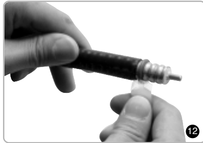
Lubricate O-ring with grease.
