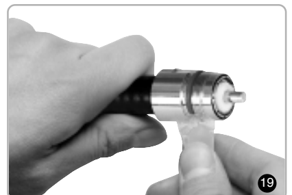
Wipe the O-ring with grease. (Well-proportioned)
