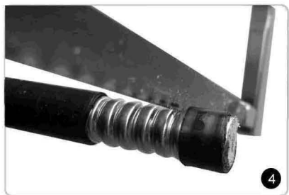
Cut the cable in the bottom of corrugation
