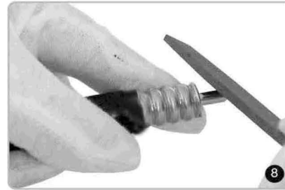
Chamfer inner conductor 1 \times 45^\circ with flat file.
